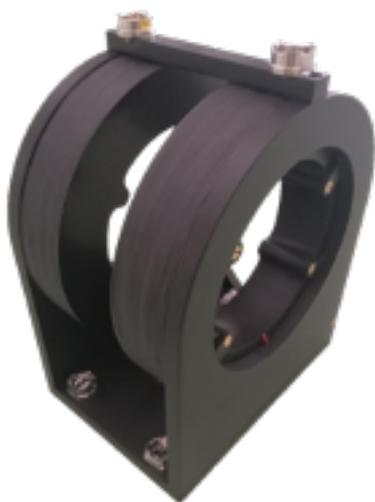
**Figure 8.** A similar HH coil developed to perform the calibration procedure in house.
