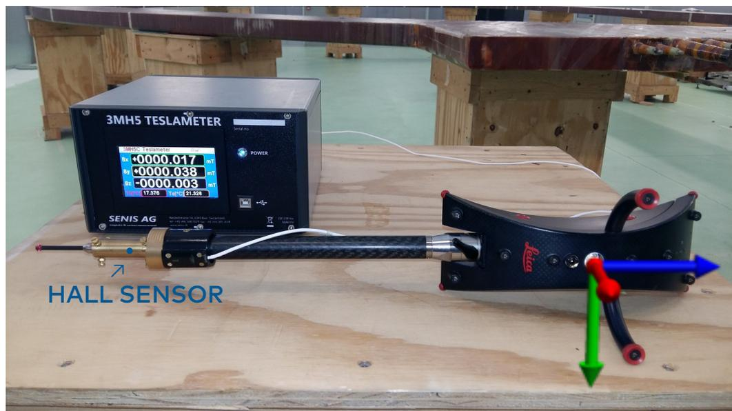
**Figure 3.** ASG integration of a SENIS Type C Hall Probe inside the stylus of a Leica T-Probe. The white cable connected to the electronics supplies the DC current to the sensor and measures the DC voltage generated by the Lorentz force. A reference frame is defined centered on the T-Probe.
